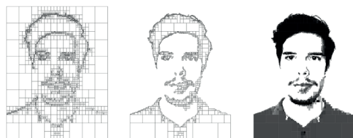
Figure 6. Quadtree of the input image (left); Outcome after of simplification process (middle); and the same quads filled with the average brightness of the corresponding area of the input image (right).
