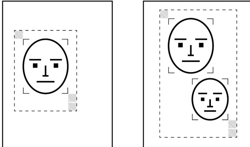
Figure 2. Calculation of the region of interest (dashed boxes) for two example scenarios according to automatically detected faces in the captured image. Each region of interest encloses the detected face(s), plus a preset margin (shaded squares).
