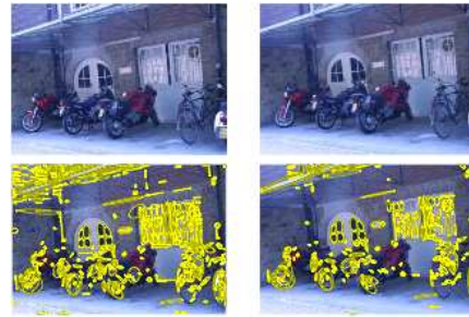
Figure 1: MSER detection (bottom row) on the first two images of the “Bikes” sequence (top row). MSErs are represented by fitted ellipses.
