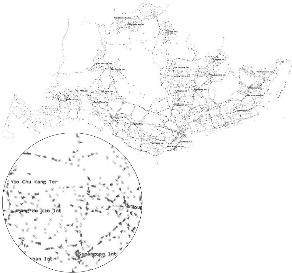
Fig. 2. Results of the clustering algorithm with a search radius of 44 meters and a minimum of 5 buses per cluster
